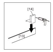
10. Apply thin beads of glass glue into the Cover Caps[14], and assemble them on both ends of the Bottom Horizontal Rail[13].
