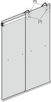
drilled holes of the Door Panel[16]. Place the bottom of Door Panel[16] into the gap between the Door Guide[10] and Bottom Horizontal Rail[13], and insert the top of Door Panel[16] into the slot of Top Horizontal Rail[8]. Install the Anti-collision Component[7] into the hole of Door Panel[16],lock and fasten it.
