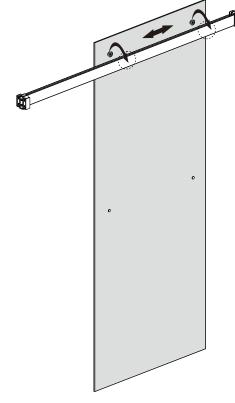
6.Install the Top Wheels[4] through the pre-drilled holes in Door Panel[5]. Stick the Top Wheels[4] in the openings of the Top Horizontal Rail[9].
