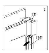
Press the Door Side Gasket[15] onto the vertical edges of the Door Panels[5&16]. Please see Fig 2 for details.
